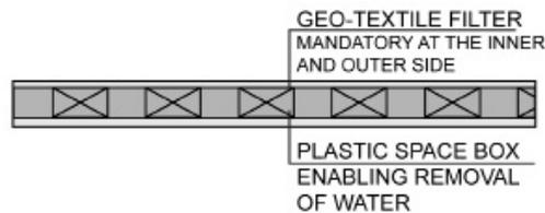
Fig. D.3 Drainage from prefabricated geo-composite:
