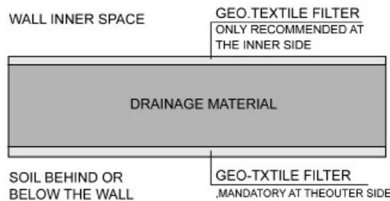
Fig. D.2 Drainage from classic drainage material:
