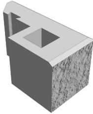
The right-hand angled element viewed to larger face surface of the block (size 400 x 200 mm) features the smaller face area at the right side (size 200 x 200 mm) see fig. a).
