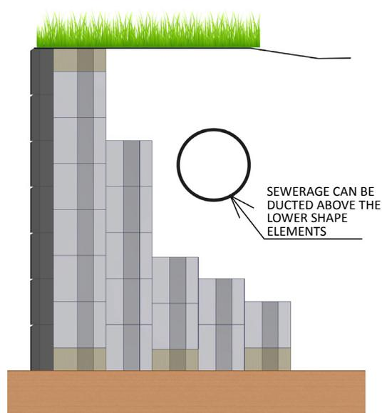
Fig. 5.4.2a Example of sewerage line:
