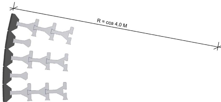
Fig. 7.1.2d Example of convex retaining wall of larger radius
