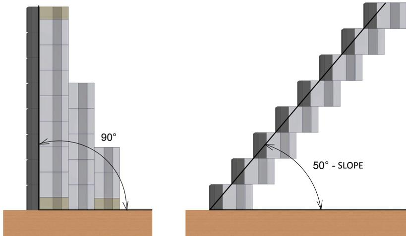
Fig. 3.1. Difference between supporting wall and escarp
