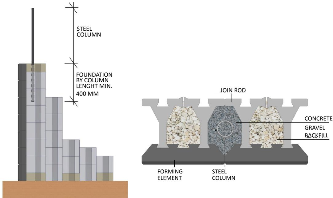
Fig. 6.7. Fitting the column to retaining walls
