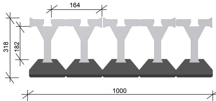
Fig. 4.5a Definition of backfill areas for determination of backfill material amount
