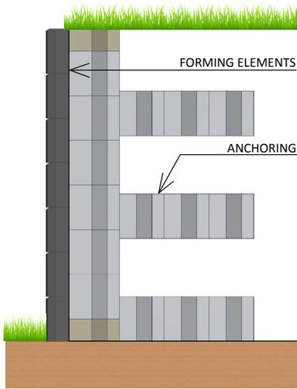
Fig. 4.2b Cross-section through wall reinforced
