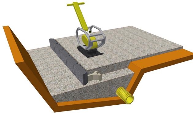
Fig. 6.2.9a Compacting of gravel bed
