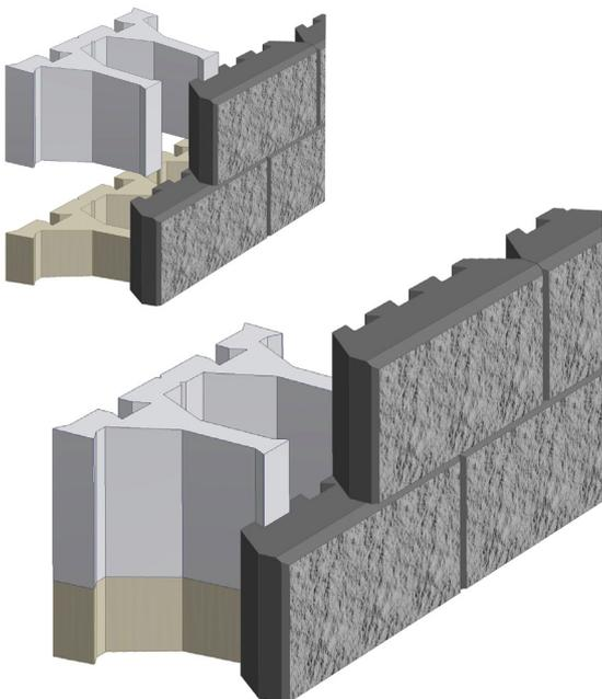
Fig. 3.2.1e Interlocked block by join rod
