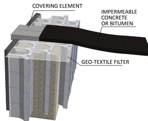
Fig. 6.6.3a Drainage trench
