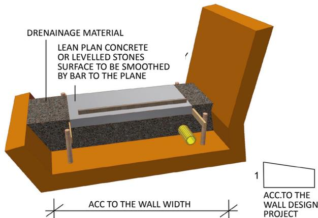
Fig. 6.2.10a Inclined gravel bed with alternative material
