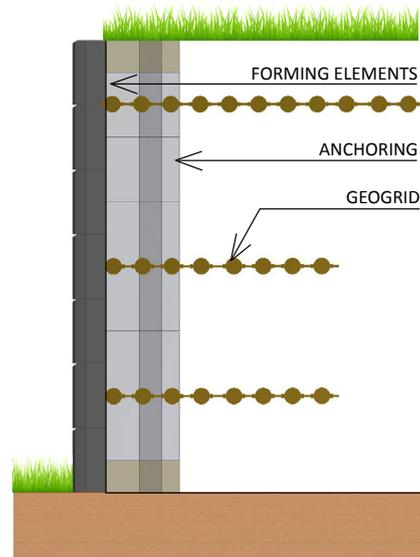
Fig. 4.2c Cross-section through wall reinforced with Geogrid
