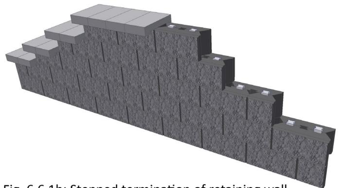
Fig. 6.6.1b: Stepped termination of retaining wall
