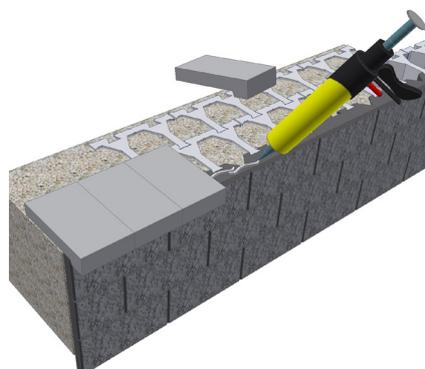
Fig. 6.6.2a Covering of retaining wall
