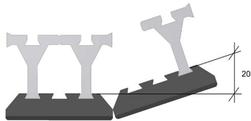
Fig. 7.1.2a Rotation angle of adjacent elements
