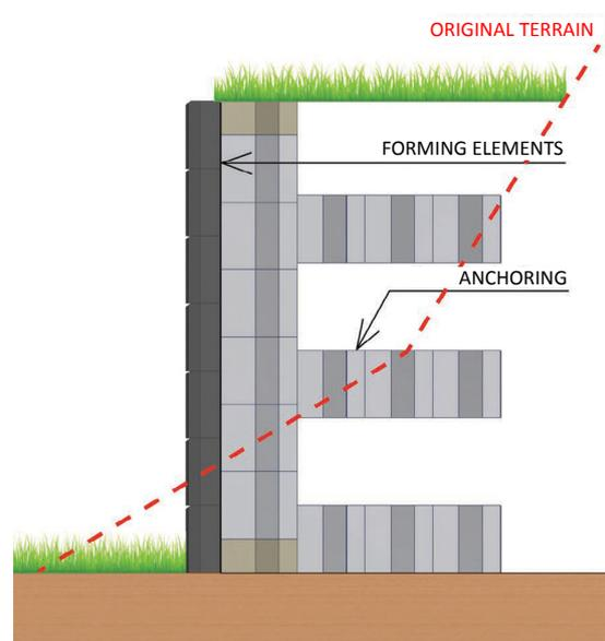
Fig. 4.2e Example of filling wall
