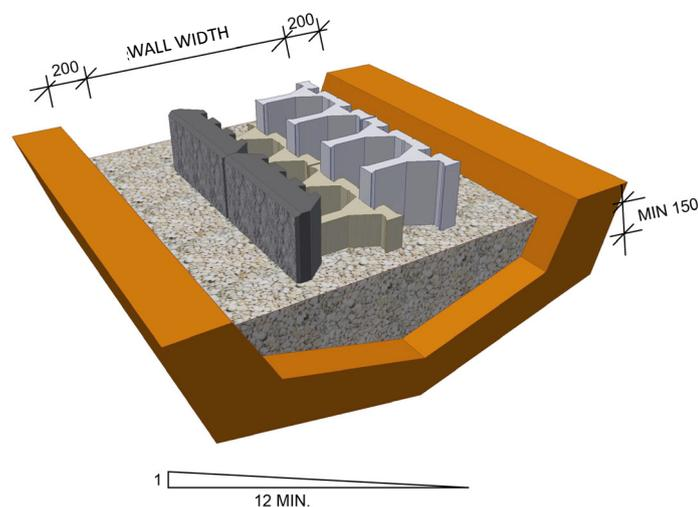
Fig. 6.2.2a Example of dugout for gravel bed
