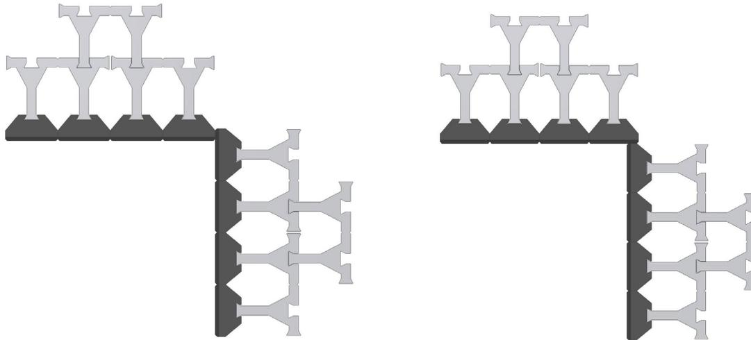
Fig. 7.2.1a Example of the wall inner corner with single anchoring
