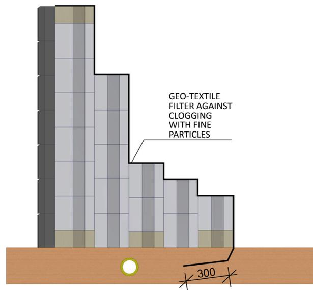
Fig. 6.2.6a Positioning of geo-textile filter
