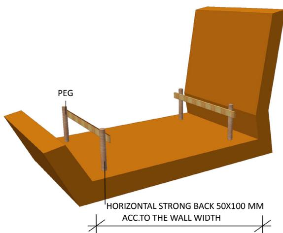
Fig. 6.2.3a Example of dugout for tilted gravel bed
