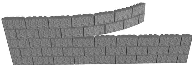
Fig. 6.6.1a: Curved termination of retaining wall
