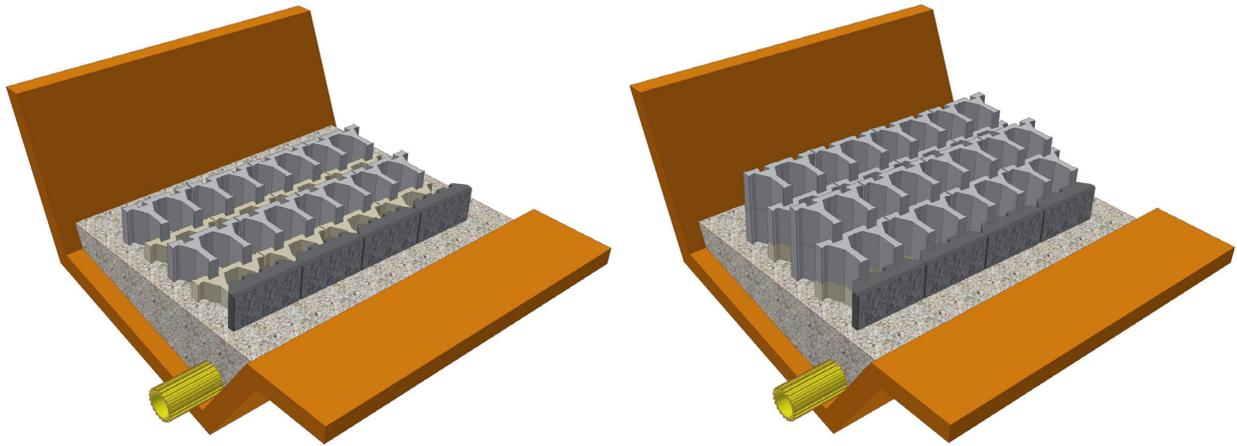
Fig. 6.3.2a: Adjusting of second and other rows of anchoring elements
