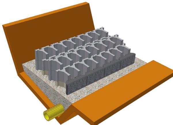
Fig. 6.4.2a: Laying of next layer of STAVOBLOCK shape elements
