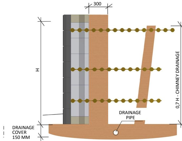
Fig. D.1 Blanket and stack drainage:
