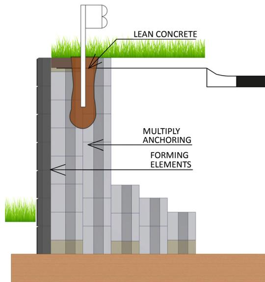
Fig. 5.4.3a Example of guard wall anchoring
