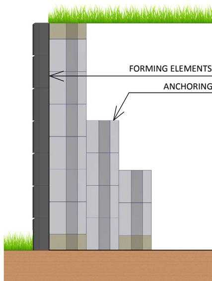
Fig. 4.2a Cross-section through modular wall
