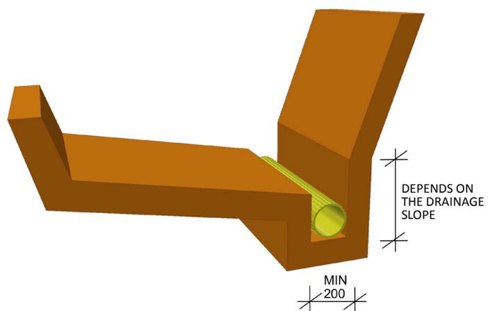
Fig. 6.2.4a Example sunk dugout for drain pipe
