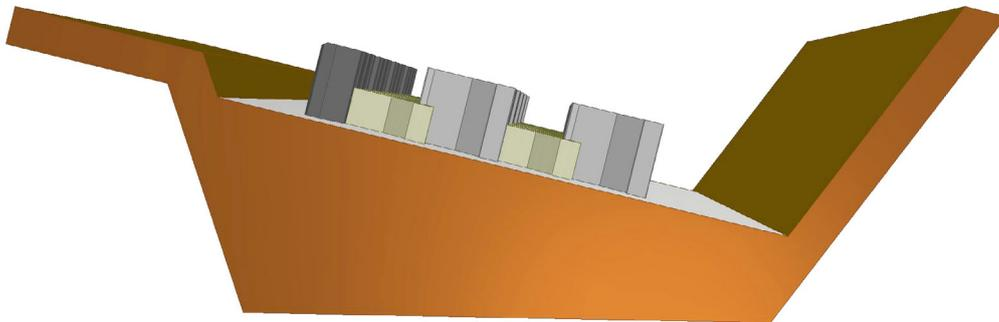
Fig. 6.3.2b: Checking of inclination angle of masonry first layer
