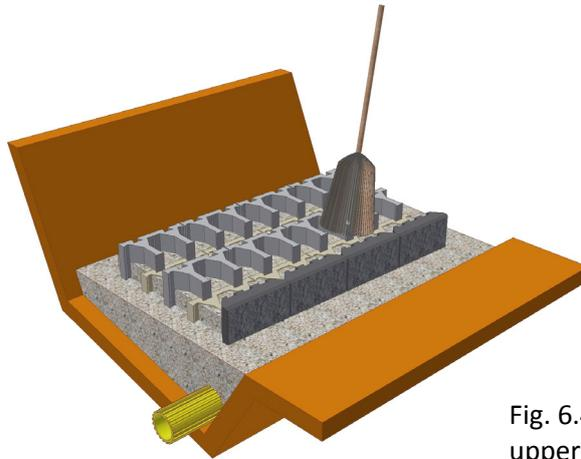
Fig. 6.4.1a: Preparation of the shape element upper face for next row of masonry
