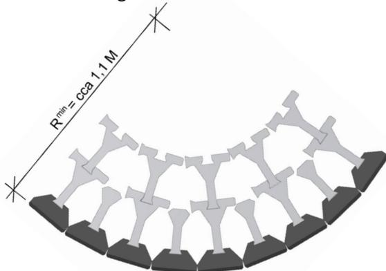
Fig. 7.1.2b Minimum radius of convex retaining wall
