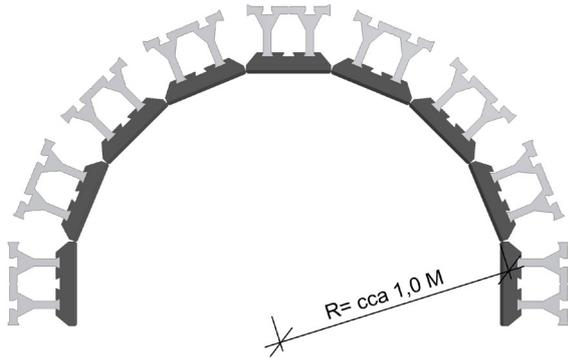
Fig. 7.1.1b Minimum radius of concave retaining wall
