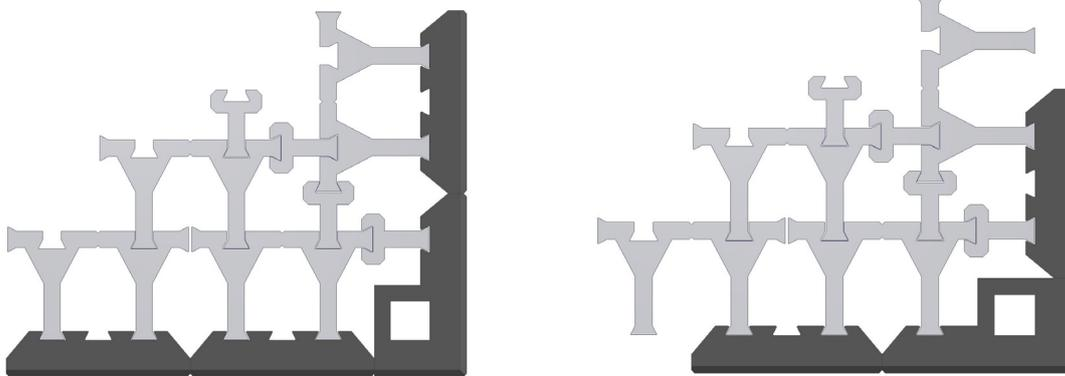
Fig. 7.2.1a Example of the wall outer corner
