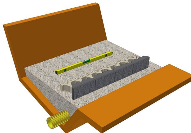
Fig. 6.3.1a Positioning of first row of basic module (face element with join rod)
