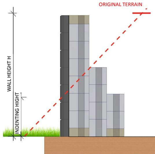
Fig. 4.2f Determination of incised ratio
