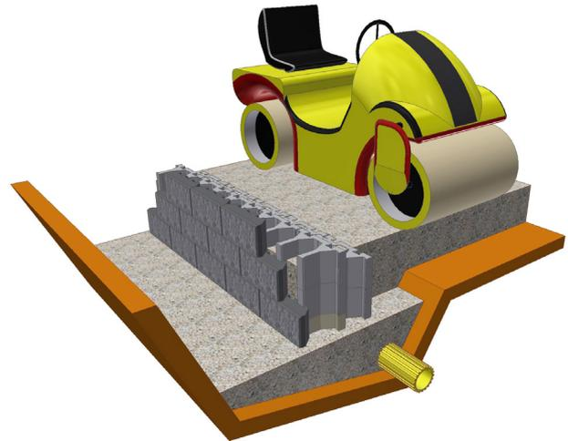
Fig. 6.4.4b: Compacting by vibrating rolls
