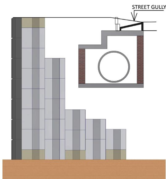
Fig. 5.4.1a Example of adaptation of modular wall to local obstacle
