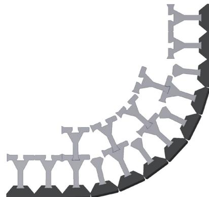
Fig. 7.1.2c Perpendicular connection of retaining wall by means of convex curve
