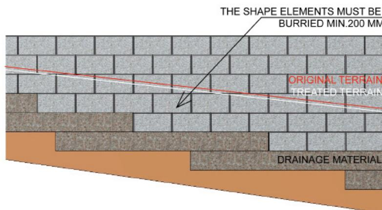
Fig. 6.3.5a: View to wall with height adjustments in laying
