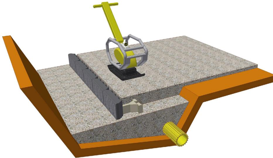
Fig. 6.3.4a: Compacting of backfill of the shape elements by means of vibration plate
