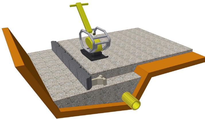
Fig. 6.4.4a: Compacting a strip of 0.8 m behind the shape elements
