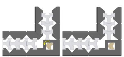
Fig.3.2.2. f - Corner elements secured with a corner peg, ideal interconnection ensured by turning the corner peg
