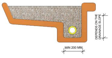
Fig. 6.2.3a Example sunk dugout for drain pipe
