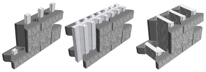
Fig. 3.1.2a Combined partition wall - from the left - width 200, 300, 400 mm
