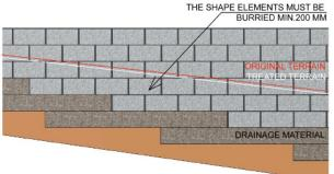
Fig. 6.3.5a: View to partition wall with height adjustments in laying
