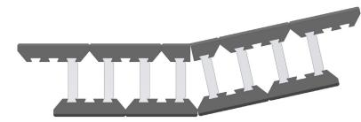
Fig. 3.2.1d Acute or obtuse angled partition wall of width 400 mm
