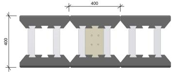
Fig. 3.2.2c Pillar 400 x 400 mm armoured, non-filled partition wall of width 400 mm
