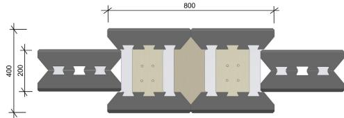
Fig. 3.2.2d Pillar 400 x 800 mm armoured, filled partition wall of width 200 mm
