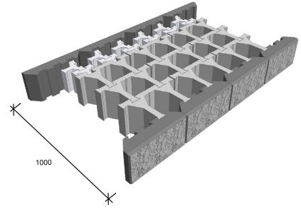
Fig. 5.2.3a: Quadruple anchoring: Face element – 3 x Join rod – 2x T-coupler – Face element Arrangement total width: + each new anchoring: + 180 mm
