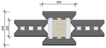
Fig. 3.2.2b Pillar 400 x 400 mm, partition wall of width 200 mm
