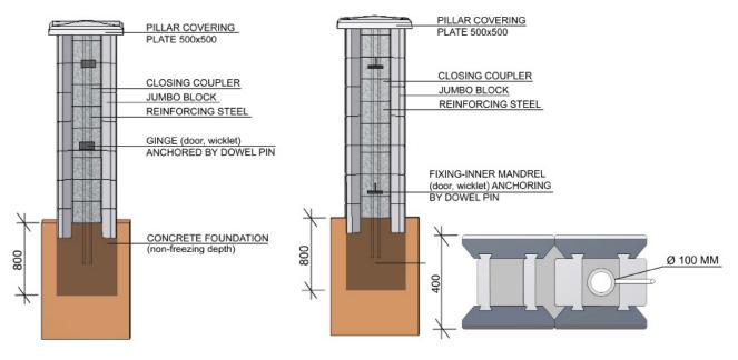
Fig. 8.3a Fixing of hinges by means of dowel pins directly to the pillar
