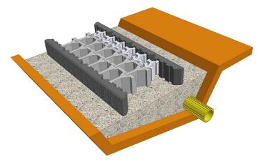
Fig. 6.3.2a: Adjustment of second and other row of the anchoring elements with positioning of the left-hand face element
