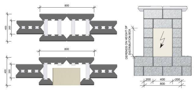
Fig. 7.1a Built-in switchboard 600 x 400 mm
