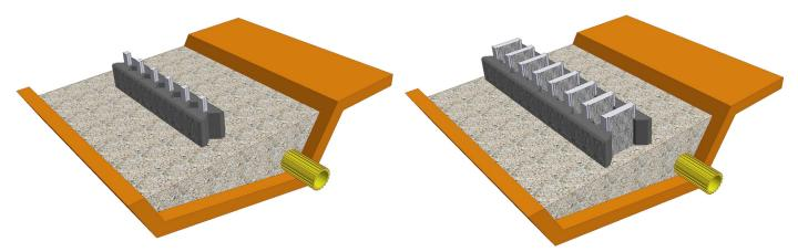
Fig. 6.3.1a,b Setting of first row of width 200/400 mm (face elements with short coupler)
