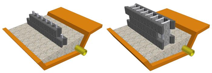
Fig. 6.4.2a: Laying of next layer of STAVOBLOCK shape elements - wall width 200/400 mm
