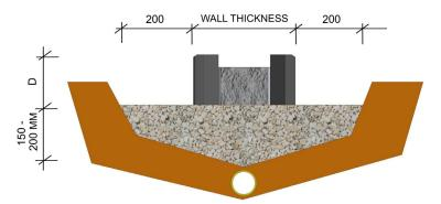
Fig. 6.2.2a Example of dugout for gravel bed
