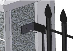
Fig. 7.2a Fixing detail - Anchoring angular piece screwed to closing coupler
