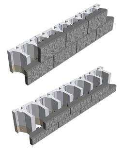
Fig. 3.2.1a Basic positioning of JUMBO blocks <u>Basic consumption per 1 m<sup>2</sup></u> from modular block: 12.5 pcs. of face elements JUMBO; 25 pcs. of join rods. <u>Basic consumption per 1 running meter</u>, height 200 mm, from modular block: 2.5 pcs. of face elements JUMBO; 5 pcs. of join rods.
