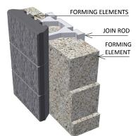
Fig. 5.3.2a Realisation of backfill at walls composed from face element and join rod (basic module)
