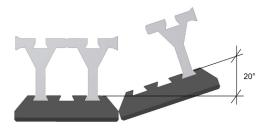
Fig. 7.1.2a Rotation angle of adjacent elements
