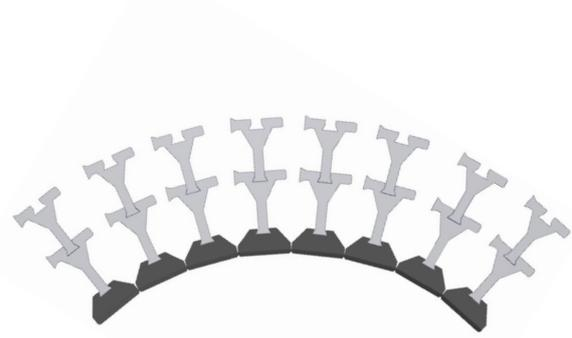
Fig. 7.1.1c Example of concave retaining wall of larger radius
