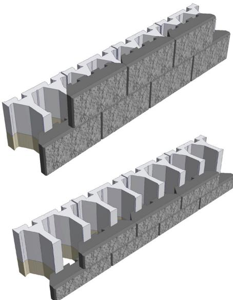
Fig. 3.2.1a Basic positioning of JUMBO blocks
