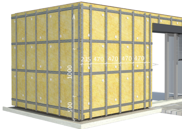
Pic.20- mounting vertical Omega bars
